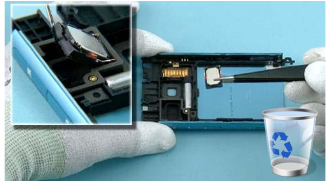
44) Release the IHF SPEAKER with the dental tool and remove it with the tweezers. Do not use the IHF SPEAKER again.
