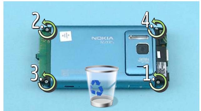
14) Unscrew the four Torx+ size 4 screws in the order shown. These screws cannot be used again. Discard them.
