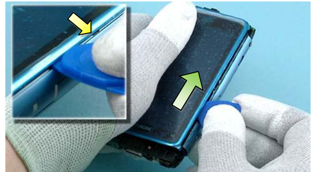
16) Release also the second clip on the other side of the phone by sliding the SRT-6 to the direction shown.
