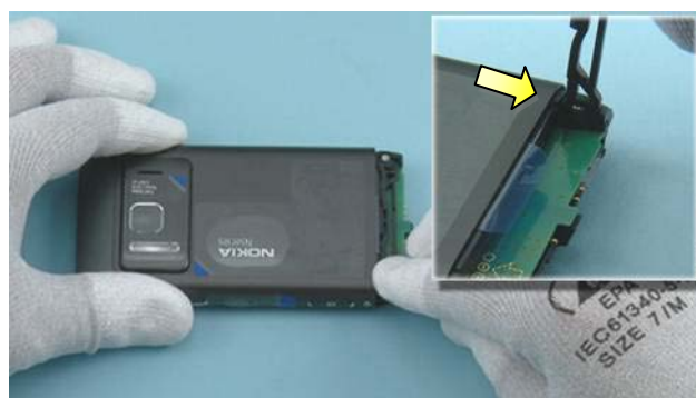
46) Place the shown end of the BATTERY LID and then lower down the other end. Note that the BATTERY PULL-OUT TAPE is left under the BATTERY LID.
