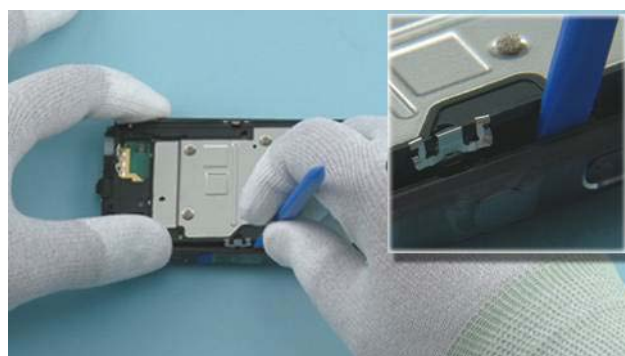
30) Use the SS-93 to spread the sides of the BODY ASSY and push down the ENGINE CHASSIS ASSY to lock the springs.
