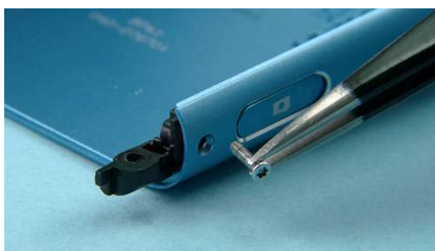
54) Remove the screw with the tweezers.
