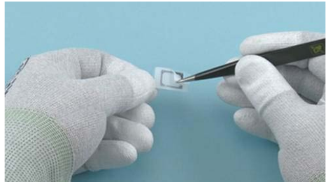
16) Remove the IHF GASKET protective film.
