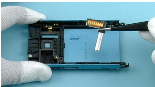
49) Remove the FLASH MODULE with the tweezers.
