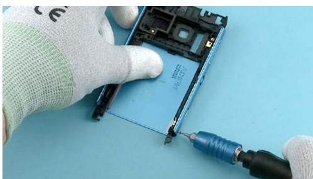
53) To release the second FIXING NUT, unscrew the Torx+ size 4 screw.
