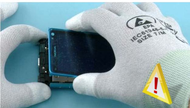
17) Carefully lift up the top side of the WINDOW ASSY to gain access to the connectors underneath. Be careful not to damage the connectors while lifting up the WINDOW ASSY!
