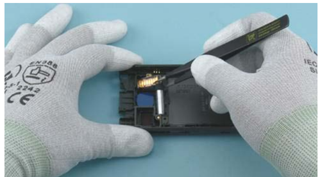
12) Place the FLASH MODULE with the tweezers.
