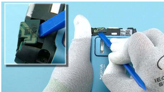
25) Release the COMBO ANTENNA with the SS-93.
